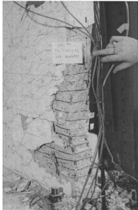
Figure A.41: ThomTW2: DS4f - TW2 damage at 2.5% drift
