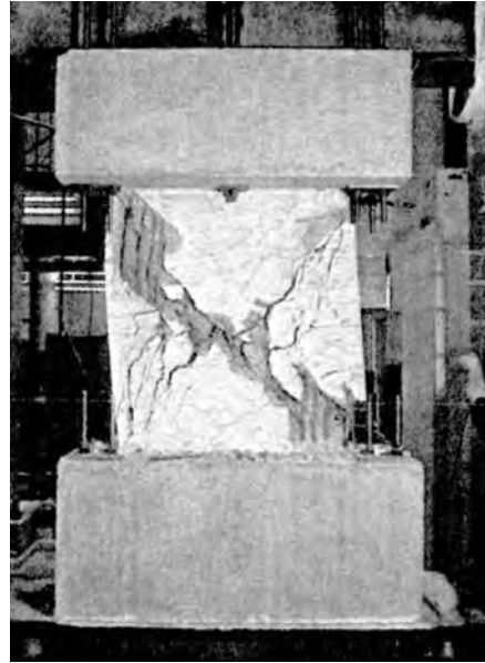
(a) Diagonal shear failure [19].
