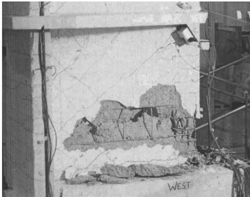
Figure A.39: ThomTW1: DS4f - TW1 damage at 1.25% drift
