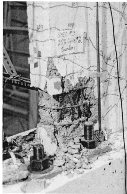
Figure A.37: ThomRW2: DS4f - RW2 damage at 2.5% drift
